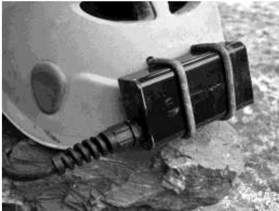
Left shows a 2 cell power pack neatly and securely fitted. I considered fancy clips etc but discounted it as we need to maintain the power pack as close to the helmet as possible whilst not adding and bulk. Power pack shown my be different to as supplied.
