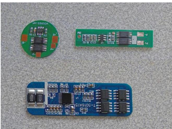
On the left can be seen a selection of Li Ion battery management modules. Top left is the kind that is mounted on the base of a single cell and enclosed within the wrapper. Top right is a type designed to manage two cells in series with an off charge voltage of 8.4V. Note the similarity between components. Both utilise a dedicated chip manufactured by Seiko Industries. These are rated at 2 amps so are mounted in pairs to handle 4 amps.
