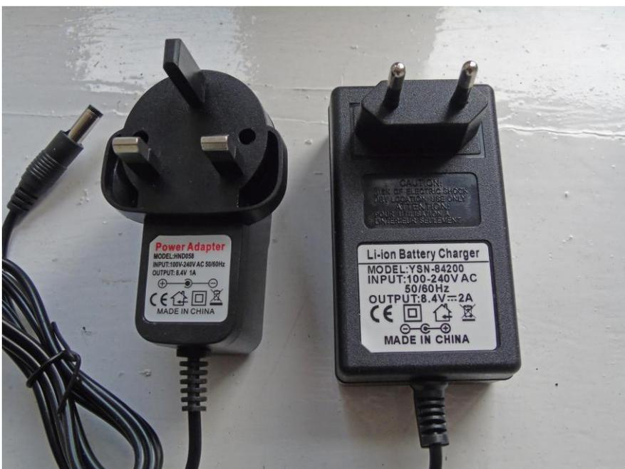
Here are two different charger types; however they both have an indicated output voltage of 8.4V which makes them suitable for charging 2 series Li Ion battery packs. However they differ in other ways. The one on the left has an output of 1 amp, so is fairly universal. A battery with multiple cell arrays will just take a fraction longer to charge. This example is not specifically
