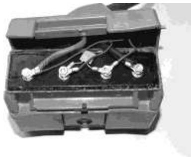
4 Cell belt mount power packs are permanently sealed and require no attention, just as the helmet packs.
